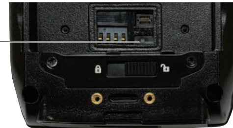
Backup Battery Switch
