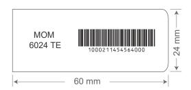
Syndicate's MOM 6024 TE is a non-transferable tamper-evident label for Mount on Metal applications demanding long read range in small form factor with a high performance permanent adhesive. Supplied in roll form as finished label and it can be encoded and printed with typical RFID printers that are capable of printing labels.
